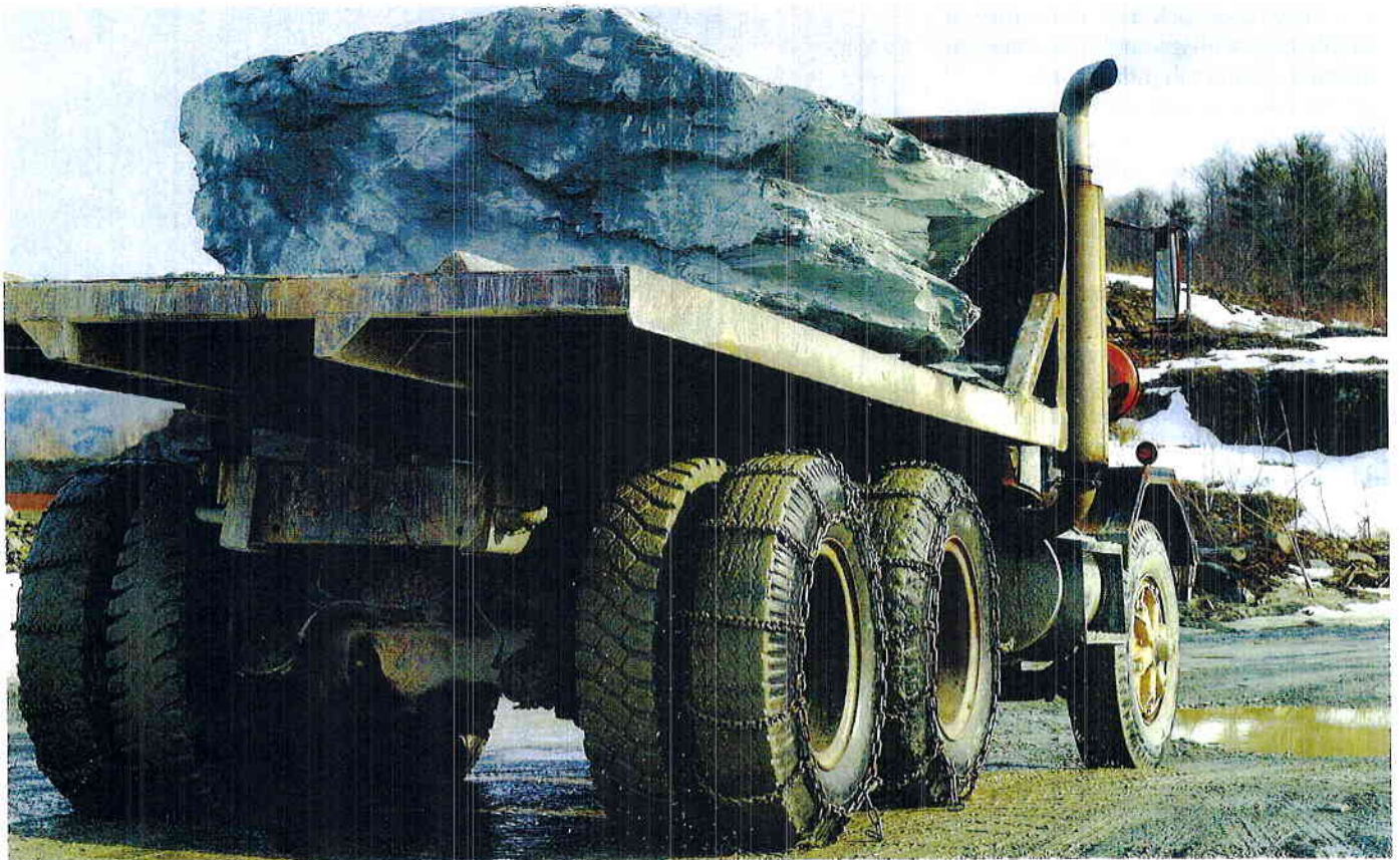
This twin-axle Autocar truck is one of several of the smaller off-road vehicles used in the quarries; the largest are 35-ton Caterpillar dump trucks that are also utilized as pit trucks. From raw stone, such as what's on the truck above, finished products have been produced that grace many prominent buildings in America, among them The Museum of Modern Art in New York City.
